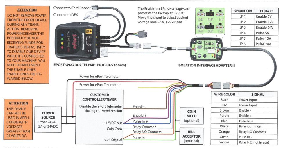
**EPORT POWER:** The Red and Black wires are used to power the ePort Telemeter. Either a 24VAC, 2A or a 24VDC, 2A power supply is recommended.
